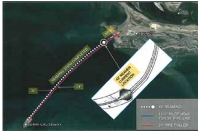
The Berri Causeway crossing showing the location of the stuck hole opener.
